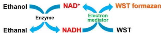
Fig. 1 Principle of NAD measurement by NAD/NADH Assay Kit-WST
